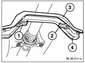
Remove bracket (1 and 2) for exhaust suspension. Remove bar (3).
