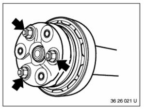
Remove flexible disk from transmission.
